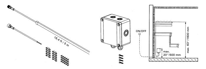
Light strip can be cut but it cannot be extended. Do not mount light strip higher than 63" from floor. If power unit is installed inside sauna room do not mount power unit higher than 20" from floor.
